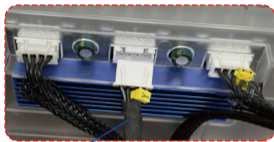
Y-Axis Motor Cable
