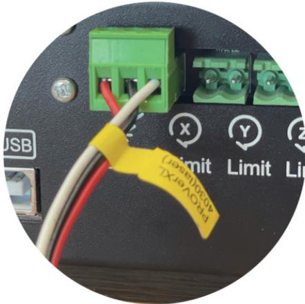
Connecting the Laser Control Module to a PROVerXL 4030 using the 3-pin cable for GND and PWM and +12v for the Laser Control Module.
