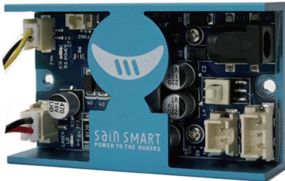
The right (as pictured) connects to your CNC via one of the 2 or 3-pin ports and the left side connects to your Laser Head and laser cooling fan. The board has a red LED to light up when power is supplied to your laser, as well as a button on the right side that toggles PWM control on and off. Take care not to press the button without taking protective measures first.
