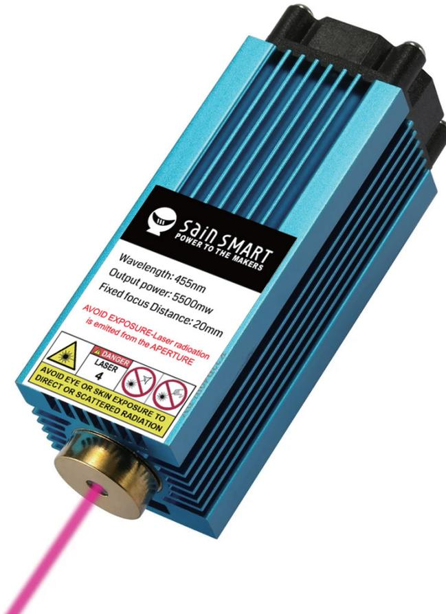
A 5.5W blue diode laser with a wavelength of 445nm. In order to ensure sufficient cooling, the laser is mounted in a heat sink, which is additionally equipped with a powerful yet quiet cooling fan. The laser has a fixed focus with a focal length of 20mm. The Laser Head is connected to the laser control unit by cables of about 30cm length. The plugs which fit into the Laser Control Module are different to ensure correct connections to the cooling fan and the Laser Diode.
