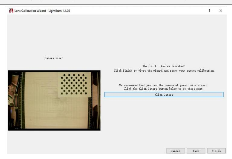
Now that the camera is calibrated, you can move on to the next step, camera alignment. This process tells LightBurn where your camera is in relation to the workspace of your machine.
