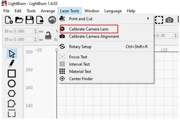
Note: The Camera Lens Calibration process involves capturing multiple images of the printed calibration image. The software examines the pattern's appearance in these images and compares it with its pre-existing understanding of the pattern's expected appearance. It then calculates the degree and form of distortion caused by the camera lens and computes a lens correction that is precise for your specific camera.
