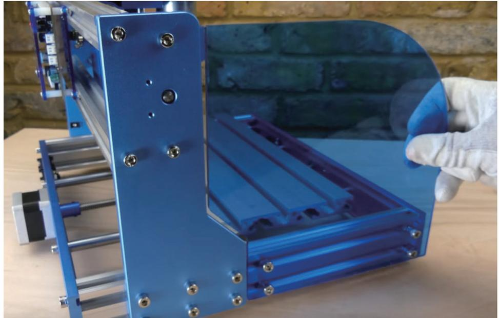
**Step 3:** Now tighten the M5 bolts to secure the baffle. Repeat the steps to install the other side.
