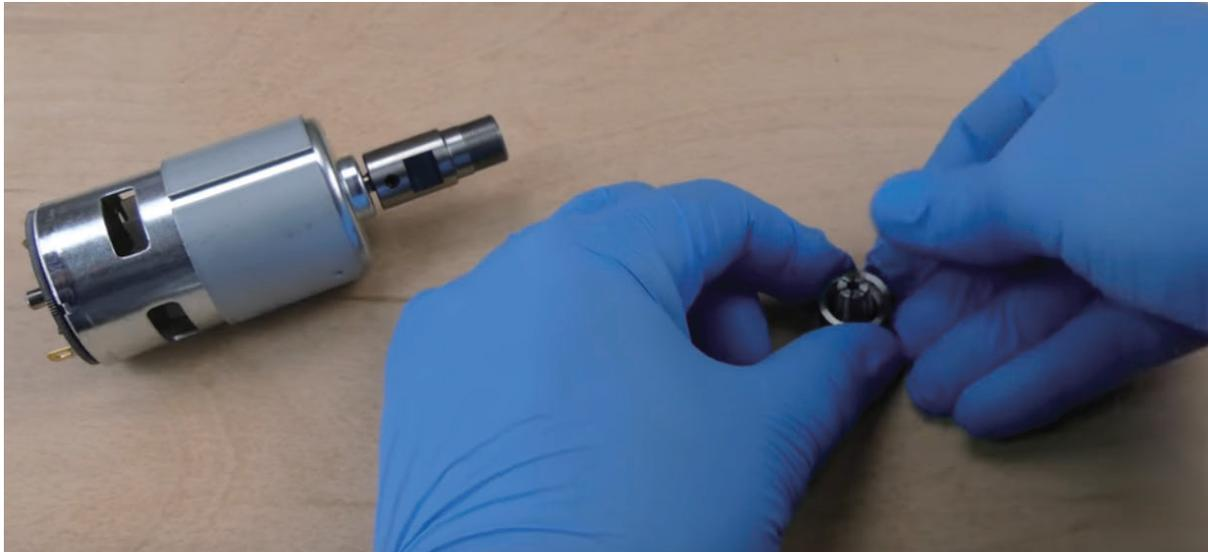
**Step 2:** Loosen the Spindle Mount Hex Screw
