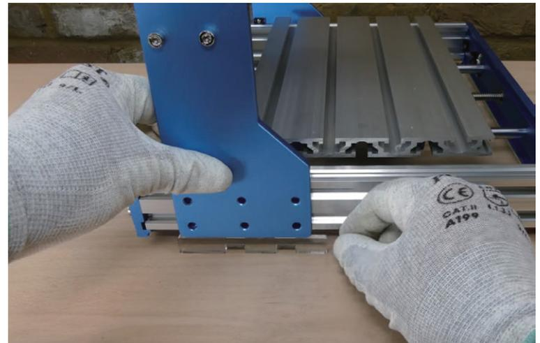
**Step 3:** Install (6) M5 14mm screws into the T-Slot nuts. Keep the screws loose until you finish the other side.
